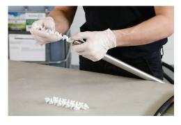
4) Position the mixing tube with the tapered end down and insert the flat end of the first element into the mixing tube stopping one inch from the top. Insert the next element into the notch of the first element and push down. Repeat for the remaining elements. 3/4 inch mixers require four elements. 1/2 inch mixers require three.
