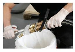
16) Holding the manifold handle in one hand, pull up on the female quick connects. Attach the manifold end to the handle and press down until it locks in place.
