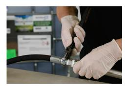
8) Attach the whip hose to the other end of the sample valve and tighten all connections.
