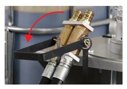
$13)\,\mathrm{Make}$  certain the manifold hand valve is closed when turning the pump on.
