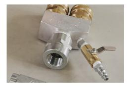
3) Remove the manifold head, mixing components and fluid gun from the solvent container and wipe off any excess solvent with a dry rag. Visually check to ensure all items are free of residue.
