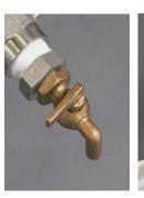
18) Make sure the drain valve and gauge valves are closed. Open the manifold handle.
