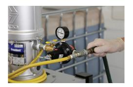
10) Attach the air hose to the air motor connector.
