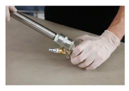
6) Attach the mixing tube to the coupler on the manifold head and tighten.
