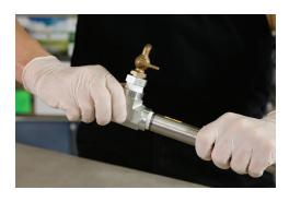
7) Attach the sample valve to the other end of the mixing tube.
