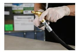
9) Complete the assembly by attaching the fluid gun to the end of the whip hose.
