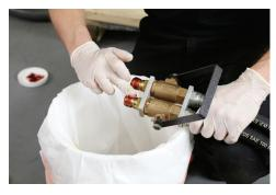
15) Apply a coat of grease to the quick connects on the manifold handle.
