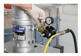
14) Turn the air supply to the air motor pump on.
