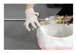
17) Attach the smart gauge to the gauge air stem.
