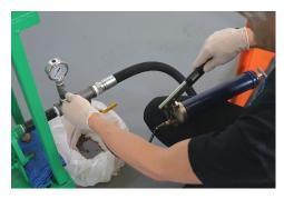
3) Run ten pumps of grease using the grease gun through the grease fitting located on the line pressure gauge.
