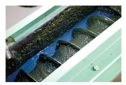
Check solvent level in mixing well and add solvent if necessary.Solvent level should be above the auger flights.
