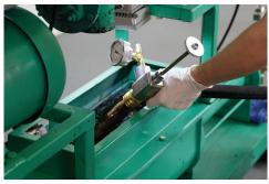
7) Place the fill hose over the mixing well and press the jog button. Allow material to circulate for 30 seconds through the system.
