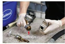
9) Remove the PSI gauge from the gun assembly. Clean the diaphragm thoroughly with a brush in 99% isopropyl alcohol. Store in a safe place.
