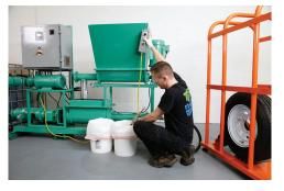
2) Place the fluid gun over an empty lined 5 gallon pail. Press and hold the "JOG" button. This will run the cavity pump only, removing the mixed flatproofing material from the mixing well, progressive cavity pump and the dispensing hose. Release the "JOG" button when the material has been purged.
