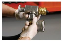
9) Attach the fluid gun and gauge assembly to the dispensing hose
