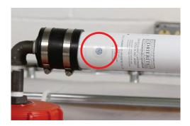
Check the inspection window on the desiccant holder. If the window is blue, proceed. If the window is pink, replace the cartridge.
