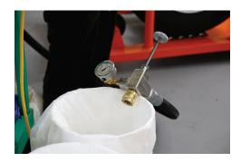
10) The Green Machine must be primed before tires can be filled. To prime the Green Machine, place the fluid gun over a waste container. Select jog P.C. on the remote and press the jog button until all the solvent has been removed from the mixing well.
