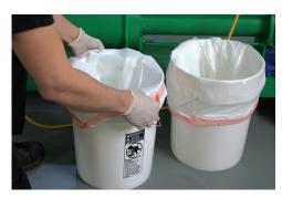
7) You will need two 5-gallon pails during operation. One pail for priming the Green Machine system on startup, and one pail for clean-up. Lining the pails with a trash bag will make disposal and reclaiming material easier.
