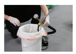
13) Press the "system start" on the remote. Allow the mixing well to fill with material. This will take about a minute. Run material into the empty pail until half full.
