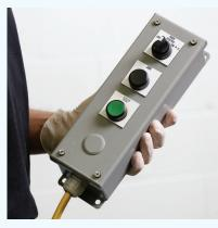
Use the remote to perform some basic functions without using the control panel, including starting and stopping.
