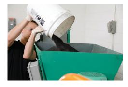
3) Check the level of the filler/grind in the hopper, add filler if needed.
