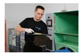
3) Used tire fill chunk should typically be cut into 12-inch sections. Inspect the chunk fill prior to depositing it into the machine to ensure no metals are present.
