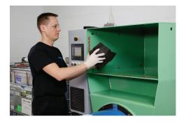
4) Fill the hopper area with chunk up to the top of the front side of the AutoFil Recycler.
