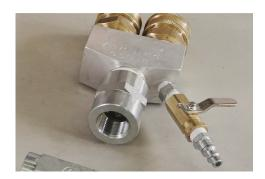
6) Remove the manifold head, mixing components and fluid gun from the solvent container and wipe off any excess solvent with a dry rag.
