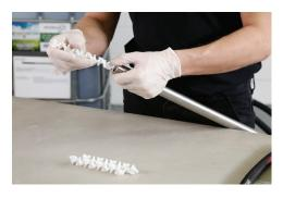
7) Using the ½ inch mixing tube, insert 3 elements. Position the mixing tube with the tapered end down and insert the flat end of the first element into the mixing tube stopping one-inch from the top. Next, insert the second element into the notch of the first element and push down. Repeat for remaining elements.
