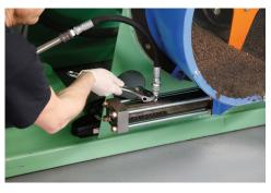
13) Attach the whip hose to the injector barrel. Tighten this connection with a wrench.
