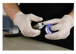
8) Dry the solvent from the ends of the mixing tube and whip hose and apply Teflon tape to the threads.
