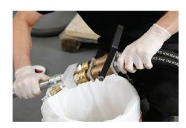
12) Holding the manifold handle in one hand, pull up on the female quick connects. Attach the manifold end to the handle and press down until it locks in place. Put the manifold in the open position.
