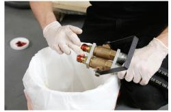
11) Apply a coat of grease to the quick connects on the manifold handle.
