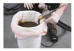
23) Hold the fill hose over a suitable container and run the mixture through the entire fill hose and gun to ensure proper flow. Here we used the foot switch to run the machine.
