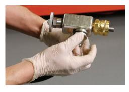
21) Connect the gun body to the other end of the hose. If the fill gun plunger isn't already attached to the gun body, attach it now.
