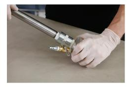
9) Attach the mixing tube to the coupler on the manifold head and tighten.
