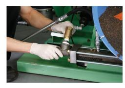
18) Connect the sample valve assembly to the injection barrel.
