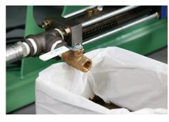
20) Place a disposable container under the sample valve assembly.
