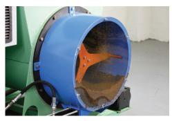
5) Turn the machine on and select Grinder. When at least half of the front hopper is filled with granulate, turn the machine off at the control panel.
